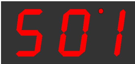
This represents Switch 01. If the number after the **S** is not **01**, press either the  $+$  or  $-$  buttons until **01** is displayed.
