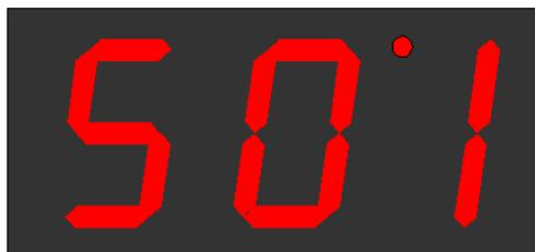
This represents Switch 01. If the number after the 5 is not 01, press either the  $+$  or  $-$  buttons until 01 is displayed.
